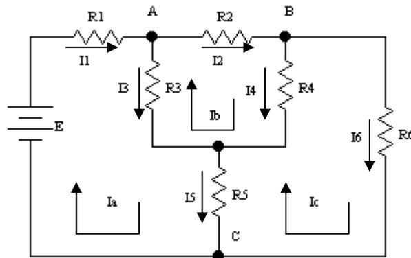
$$\begin{cases} \text{maglia a} & E = R_1 I_a + R_3 (I_a - I_b) + R_5 (I_a - I_c) \\ \text{maglia b} & 0 = R_2 I_b + R_3 (I_b - I_a) + R_4 (I_b - I_c) \\ \text{maglia c} & 0 = R_4 (I_c - I_b) + R_5 (I_c - I_a) + R_6 I_c \end{cases} \Rightarrow$$
