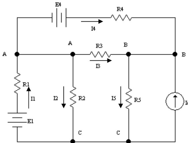
$$E_1 = 6V \quad ; \quad E_4 = 4V \quad ; \quad I_0 = 2mA$$
