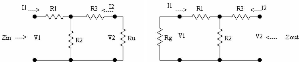
$$\bar{Z}_{in} = \frac{V_1}{I_1} = R_1 + \frac{R_2(R_3 + R_u)}{R_2 + R_3 + R_u}$$
