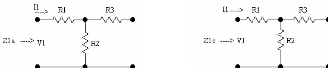
$$\begin{cases} Z_{1a} = \frac{V_1}{I_1} \Big|_{I_2=0} = R_1 + R_2 \\ Z_{1c} = \frac{V_1}{I_1} \Big|_{V_2=0} = R_1 + \frac{R_2 R_3}{R_2 + R_3} \end{cases} \Rightarrow Z_{i1} = \sqrt{Z_{1a} \cdot Z_{1c}} = \sqrt{(R_1 + R_2) \left( R_1 + \frac{R_2 R_3}{R_2 + R_3} \right)}$$
