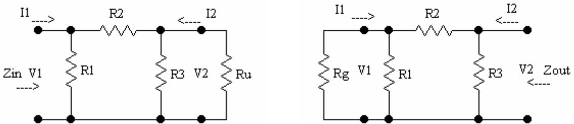
$$R_{2u} = R_2 + R_3 // R_u = R_2 + \frac{R_3 R_u}{R_3 + R_u} \Rightarrow Z_{in} = \frac{V_1}{I_1} = \frac{R_1 R_{2u}}{R_1 + R_{2u}}$$
