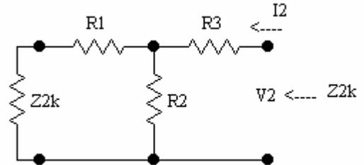
$$Z_{2k} = R_1 + \frac{R_2(R_3 + Z_{2k})}{R_2 + R_3 + Z_{2k}} \Rightarrow Z_{2k}(R_2 + R_3) + Z_{2k}^2 = R_1(R_2 + R_3) + R_1 Z_{2k} + R_2 R_3 + R_2 Z_{2k} \Rightarrow$$
