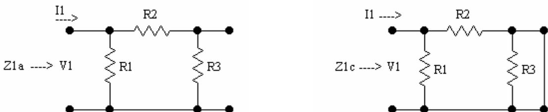
$$\left\{ \begin{aligned} Z_{1a} &= \frac{V_1}{I_1} \Big|_{I_2=0} = \frac{R_1(R_2 + R_3)}{R_1 + R_2 + R_3} \\ Z_{1c} &= \frac{V_1}{I_1} \Big|_{V_2=0} = \frac{R_1 R_2}{R_1 + R_2} \end{aligned} \right. \Rightarrow Z_{1l} = \sqrt{Z_{1a} \cdot Z_{1c}} = \sqrt{\frac{R_1(R_2 + R_3)}{R_1 + R_2 + R_3} \cdot \frac{R_1 R_2}{R_1 + R_2}}$$
