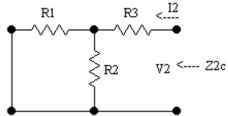
$$\begin{cases} Z_{2a} = \frac{V_2}{I_2} \Big|_{I_1=0} = R_2 + R_3 \\ Z_{2c} = \frac{V_2}{I_2} \Big|_{V_1=0} = R_3 + \frac{R_1 R_2}{R_1 + R_2} \end{cases} \Rightarrow Z_{i2} = \sqrt{Z_{2a} \cdot Z_{2c}} = \sqrt{(R_2 + R_3) \left( R_3 + \frac{R_1 R_2}{R_1 + R_2} \right)}$$
