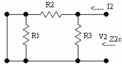
$$\left\{ \begin{aligned} Z_{2a} &= \frac{V_2}{I_2} \Big|_{I_1=0} = \frac{R_3(R_1 + R_2)}{R_1 + R_2 + R_3} \\ Z_{2c} &= \frac{V_2}{I_2} \Big|_{V_1=0} = \frac{R_2 R_3}{R_2 + R_3} \end{aligned} \right. \Rightarrow Z_{2l} = \sqrt{Z_{2a} \cdot Z_{2c}} = \sqrt{\frac{R_3(R_1 + R_2)}{R_1 + R_2 + R_3} \cdot \frac{R_2 R_3}{R_2 + R_3}}$$
