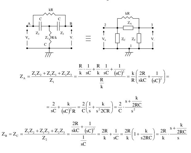
$$V_{-} = \frac{Z_{C}}{Z_{A} // kR + Z_{C}} V_{o} \implies B = \frac{V_{-}}{V_{o}} = \frac{Z_{C}}{Z_{A} // kR + Z_{C}}$$
