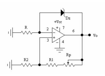
Dati: I.C. TL081;  $V_{CC} = 12V$ ;  $V_Z = 4.7V$ ;  $I_Z = 4mA$ ;  $V_0 = 6V > V_z$ .
