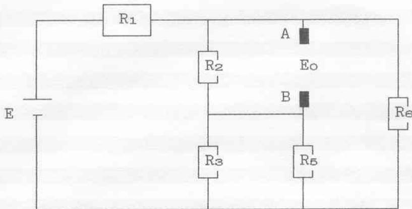
$$R_{25} = R_2 + R_{35} = 6,8 \cdot 10^3 + 2,08 \cdot 10^3 = 8,88 \text{ k}\Omega$$
