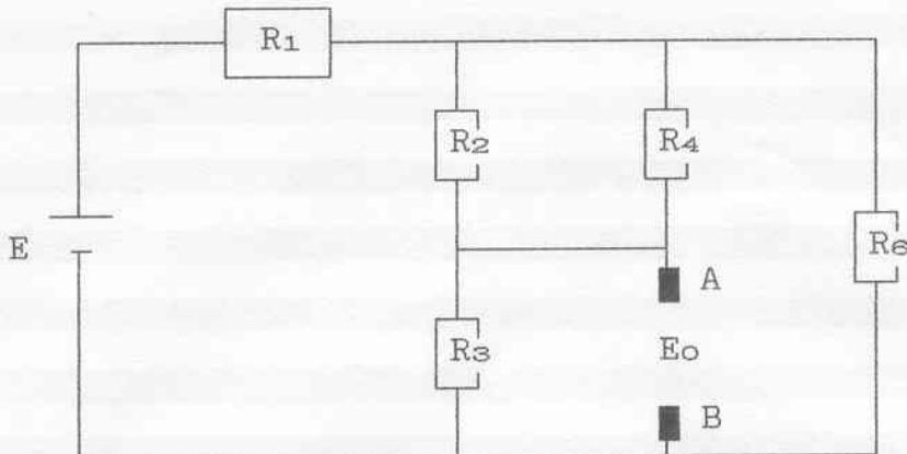
$$R_{24} = \frac{R_2 * R_4}{R_2 + R_4} = \frac{1*10^3 * 6,8*10^3}{1*10^3 + 6,8*10^3} = 0,87 \text{ k}\Omega$$
