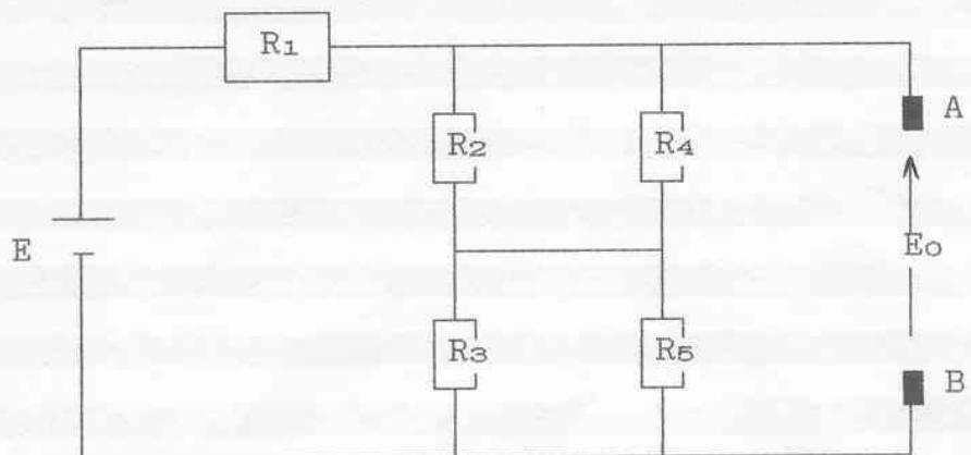
$$E_o = \frac{R_{25}}{R_1 + R_{25}} * E = \frac{2,51 \cdot 10^3}{3,3 \cdot 10^3 + 2,51 \cdot 10^3} * 14,17 = 6,12 \text{ V}$$
