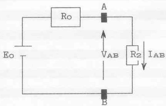
$$I_{AB} = \frac{E_o}{R_o + R_2} = \frac{1,63}{2,09*10^3 + 1*10^3} = 0,527 \text{ mA}$$
