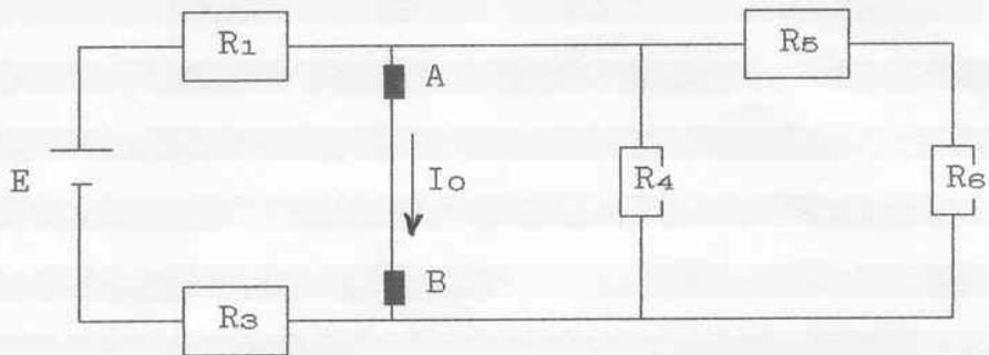
$$I_o = \frac{E}{R_1 + R_3} = \frac{9,63}{6,8*10^3 + 5,6*10^3} = 0,78 \text{ mA}$$
