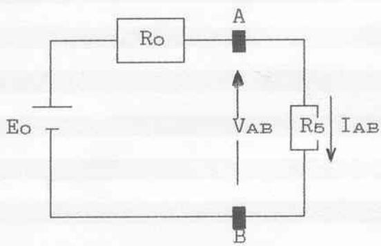
$$I_{AB} = \frac{E_O}{R_O + R_5} = \frac{21,79}{1,26*10^3 + 4,7*10^3} = 3,66 \text{ mA}$$
