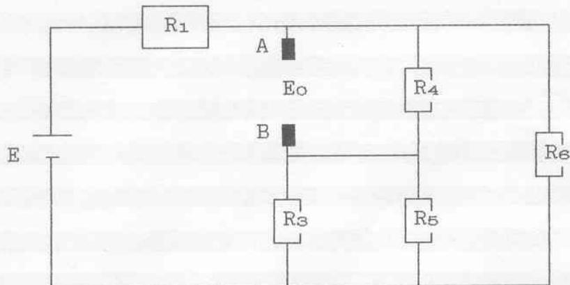
$$R_{35} = \frac{R_3 * R_5}{R_3 + R_5} = \frac{3,3*10^3 * 6,8*10^3}{3,3*10^3 + 6,8*10^3} = 2,22 \text{ k}\Omega$$
