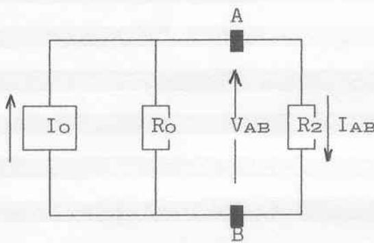
$$R_{o2} = \frac{R_o * R_2}{R_o + R_2} = \frac{1,98*10^3 * 2,2*10^3}{1,98*10^3 + 2,2*10^3} = 1,04 \text{ k}\Omega$$
