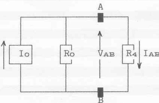
$$R_{o4} = \frac{R_o * R_4}{R_o + R_4} = \frac{2,32*10^3 * 6,8*10^3}{2,32*10^3 + 6,8*10^3} = 1,73 \text{ k}\Omega$$
