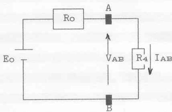
$$I_{AB} = \frac{E_o}{R_o + R_4} = \frac{1,62}{1,975*10^3 + 4,7*10^3} = 0,24 \text{ mA}$$
