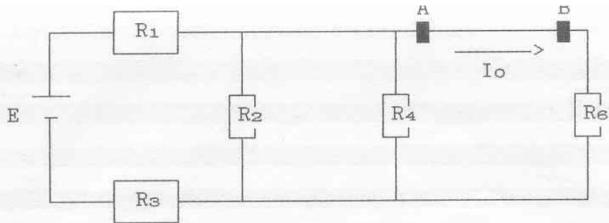
$$R_{26} = \frac{R_6 * R_{24}}{R_6 + R_{24}} = \frac{1*10^3 * 2,78*10^3}{1*10^3 + 2,78*10^3} = 0,735 \text{ k}\Omega$$
