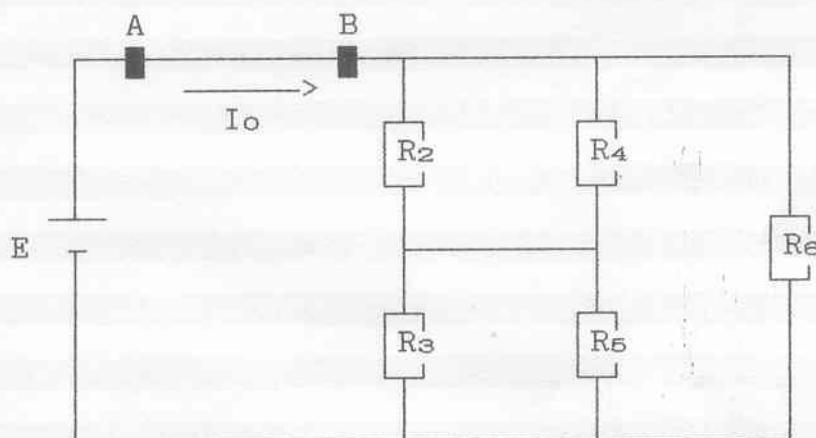
$$R_{24} = \frac{R_2 * R_4}{R_2 + R_4} = \frac{2,2*10^3 * 1*10^3}{2,2*10^3 + 1*10^3} = 0,69 \text{ k}\Omega$$
