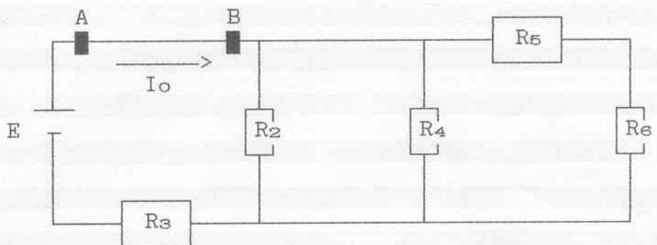
$$R_{36} = R_{26} + R_3 = 1,43 \cdot 10^3 + 1 \cdot 10^3 = 2,43 \text{ k}\Omega$$
