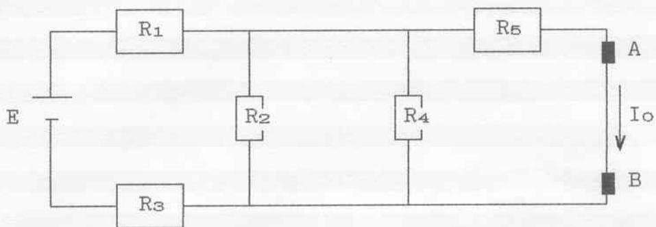
$$R_{25} = \frac{R_{24} * R_5}{R_{24} + R_5} = \frac{1,32*10^3 * 6,8*10^3}{1,32*10^3 + 6,8*10^3} = 1,1 \text{ k}\Omega$$
