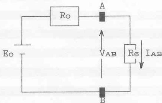
$$I_{AB} = \frac{E_o}{R_o + R_s} = \frac{1,97}{7,88*10^3 + 5,6*10^3} = 0,146 \text{ mA}$$
