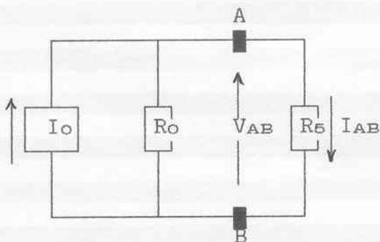
$$R_{o5} = \frac{R_o * R_5}{R_o + R_5} = \frac{3,05*10^3 * 3,3*10^3}{3,05*10^3 + 3,3*10^3} = 1,585 \text{ k}\Omega$$
