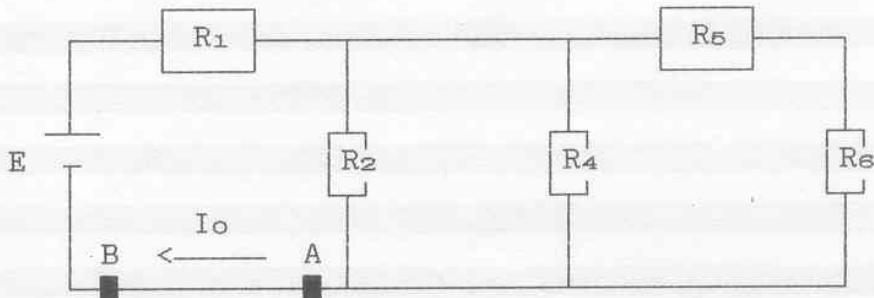
$$R_{24} = \frac{R_2 * R_4}{R_2 + R_4} = \frac{3,3*10^3 * 6,8*10^3}{3,3*10^3 + 6,8*10^3} = 2,22 \text{ k}\Omega$$
