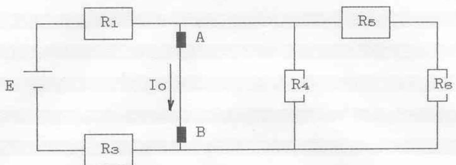
$$I_o = \frac{E}{R_1 + R_3} = \frac{533,4}{3,3 \cdot 10^3 + 2,2 \cdot 10^3} = 96,96 \text{ mA}$$
