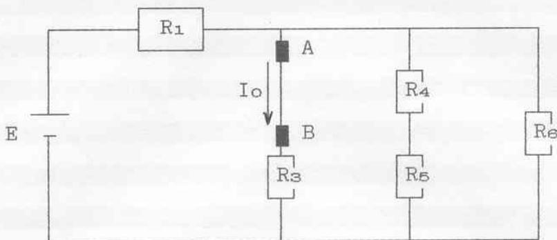
$$R_{36} = \frac{R_3 * R_{46}}{R_3 + R_{46}} = \frac{1*10^3 * 3,29*10^3}{1*10^3 + 3,29*10^3} = 0,767 \text{ k}\Omega$$
