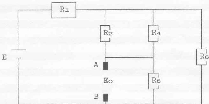
$$R_{24} = \frac{R_2 * R_4}{R_2 + R_4} = \frac{1*10^3 * 4,7*10^3}{1*10^3 + 4,7*10^3} = 0,82 \text{ K}\Omega$$
