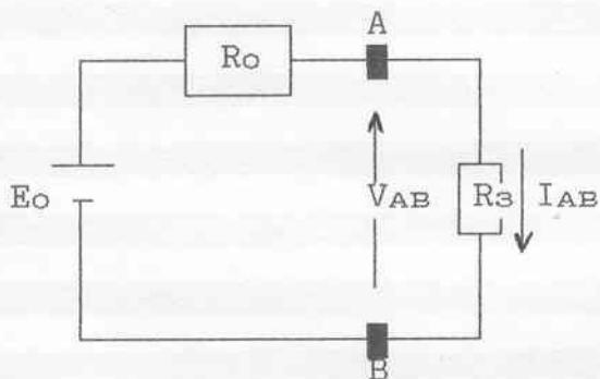
$$I_{AB} = \frac{E_o}{R_o + R_3} = \frac{8,85}{6,91*10^3 + 4,7*10^3} = 0,762 \text{ mA}$$
