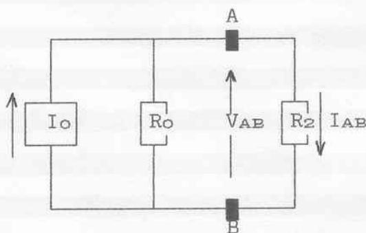
$$R_{o2} = \frac{R_o * R_2}{R_o + R_2} = \frac{2,34*10^3 * 6,8*10^3}{2,34*10^3 + 6,8*10^3} = 1,74 \text{ k}\Omega$$
