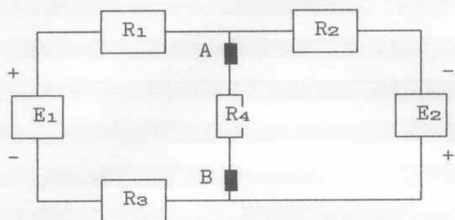
$$\begin{aligned} E_1 &= 12 \text{ V} & E_2 &= 8 \text{ V} \\ R_1 &= 2 \text{ k}\Omega & R_2 &= 4 \text{ k}\Omega \\ R_3 &= 1 \text{ k}\Omega & R_4 &= 4 \text{ k}\Omega \end{aligned}$$
