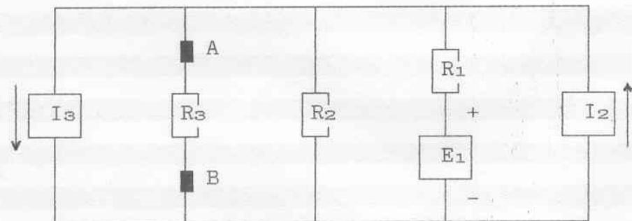
$$E_1 = 12 \text{ V} ; \quad I_2 = 3 \text{ mA} ; \quad I_3 = 1 \text{ mA} ; \quad R_1 = 2 \text{ k}\Omega$$
