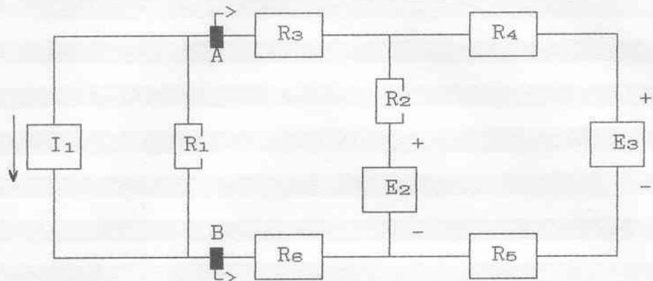
$$I_1 = 5 \text{ mA} ; E_2 = 6 \text{ V} ; E_s = 4 \text{ V} ; R_1 = 1,6 \text{ k}\Omega ; R_2 = 1 \text{ k}\Omega$$
