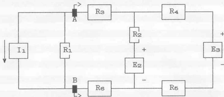
$$I_1 = 5 \text{ mA} ; E_2 = 6 \text{ V} ; E_3 = 4 \text{ V} ; R_1 = 1,6 \text{ k}\Omega ; R_2 = 1 \text{ k}\Omega \\ R_3 = 2 \text{ k}\Omega ; R_4 = 1,5 \text{ k}\Omega ; R_5 = 2,5 \text{ k}\Omega ; R_6 = 3 \text{ k}\Omega$$
