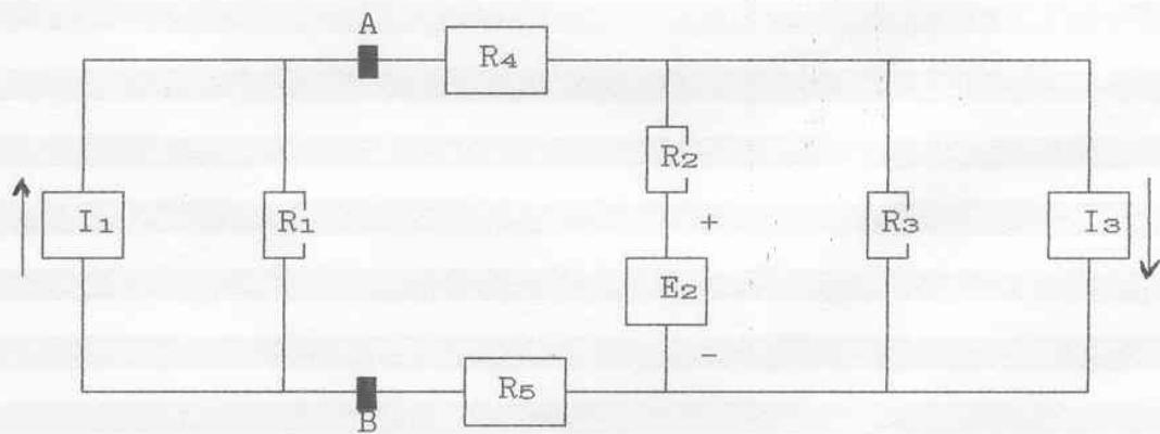
$$I_1 = 6 \text{ mA} ; E_2 = 8 \text{ V} ; I_3 = 3 \text{ mA} ; R_1 = 1 \text{ k}\Omega$$
