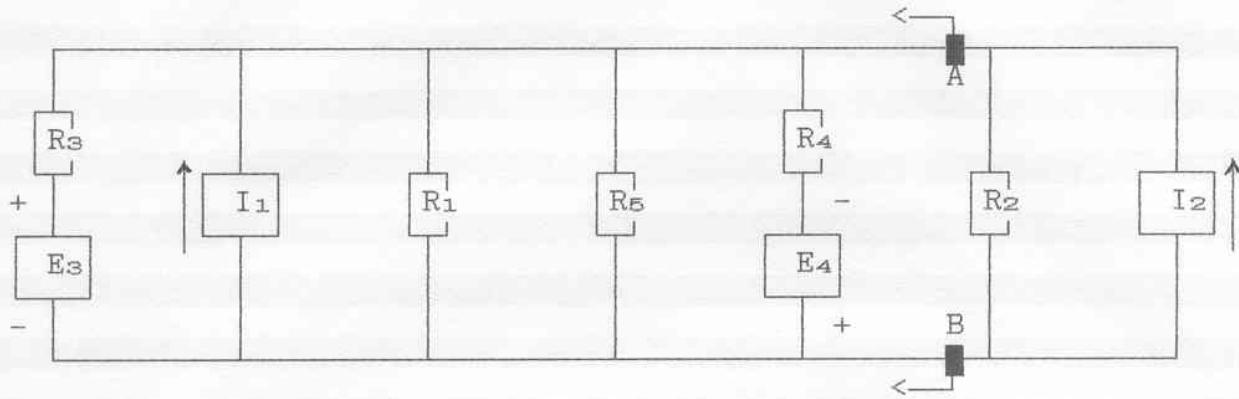
$$I_1 = 6 \text{ mA} ; \quad I_2 = 10 \text{ mA} ; \quad E_3 = 8 \text{ V} ; \quad E_4 = 10 \text{ V}$$
