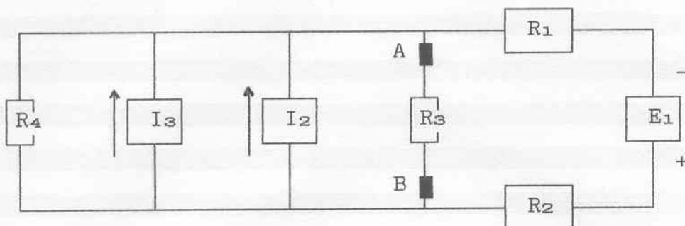
$$E_1 = 12 \text{ V} ; \quad I_2 = 2 \text{ mA} ; \quad I_3 = 3 \text{ mA} ; \quad R_1 = 5 \text{ k}\Omega$$
