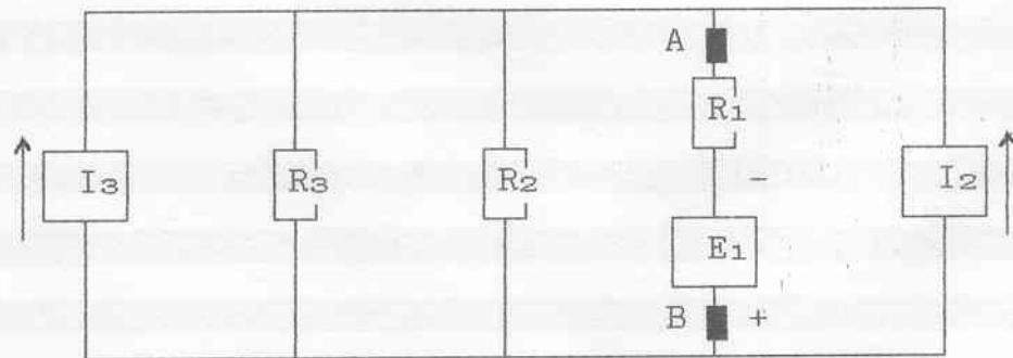
$$E_1 = 12 \text{ V} ; \quad I_2 = 4 \text{ mA} ; \quad I_3 = 2 \text{ mA} ; \quad R_1 = 10 \text{ k}\Omega$$
