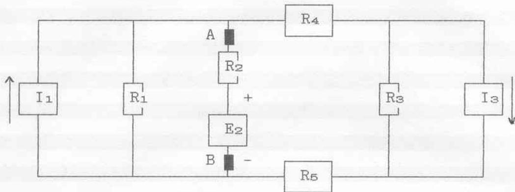
$$I_1 = 6 \text{ mA} ; E_2 = 6 \text{ V} ; I_3 = 8 \text{ mA} ; R_1 = 1,5 \text{ k}\Omega$$
