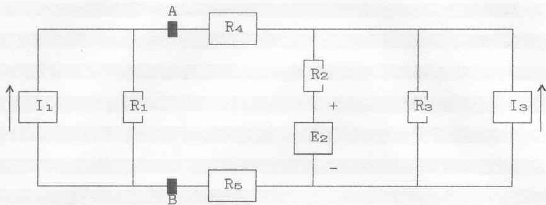
$$I_1 = 5 \text{ mA} ; E_2 = 10 \text{ V} ; I_3 = 2 \text{ mA} ; R_1 = 2 \text{ k}\Omega$$
