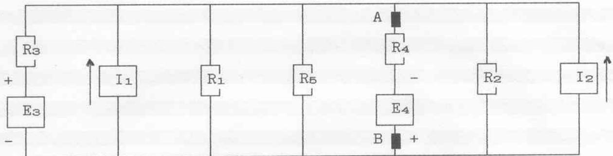
$$I_1 = 6 \text{ mA} ; \quad I_2 = 10 \text{ mA} ; \quad E_3 = 8 \text{ V} ; \quad E_4 = 10 \text{ V}$$
