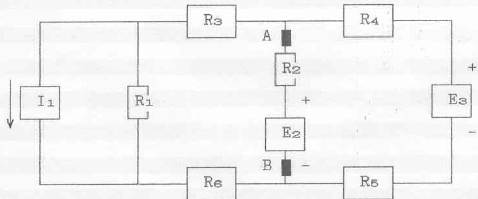
$$I_1 = 5 \text{ mA} ; E_2 = 6 \text{ V} ; E_s = 4 \text{ V} ; R_1 = 1,6 \text{ k}\Omega ; R_2 = 1 \text{ k}\Omega$$
