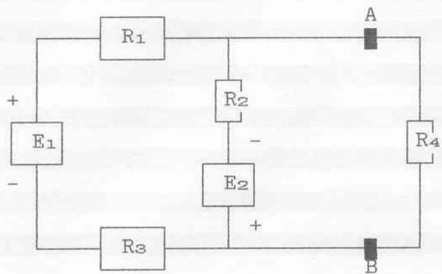
$$\begin{aligned} E_1 &= 16 \text{ V} & E_2 &= 8 \text{ V} \\ R_1 &= 2 \text{ k}\Omega & R_2 &= 2 \text{ k}\Omega \\ R_3 &= 1 \text{ k}\Omega & R_4 &= 5 \text{ k}\Omega \end{aligned}$$
