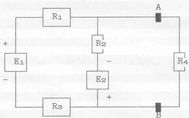
$$\begin{aligned} E_1 &= 24 \text{ V} & E_2 &= 12 \text{ V} \\ R_1 &= 1 \text{ k}\Omega & R_2 &= 1 \text{ k}\Omega \\ R_3 &= 1,5 \text{ k}\Omega & R_4 &= 3 \text{ k}\Omega \end{aligned}$$
