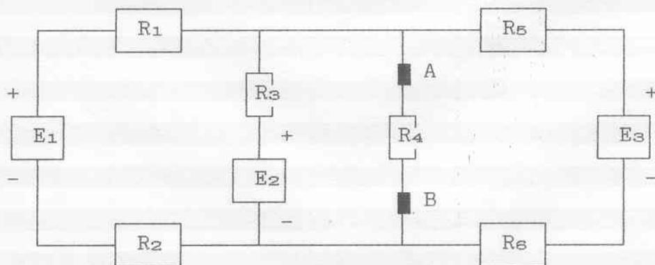
$$1.- \quad E_1 = E_2 = E_3 = 10 \text{ V} ; \quad R_1 = R_3 = R_5 = 2 \text{ k}\Omega ; \quad R_2 = R_4 = R_6 = 3 \text{ k}\Omega$$
