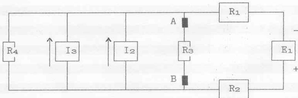
$$E_1 = 12 \text{ V} ; I_2 = 2 \text{ mA} ; I_3 = 3 \text{ mA} ; R_1 = 5 \text{ k}\Omega$$
