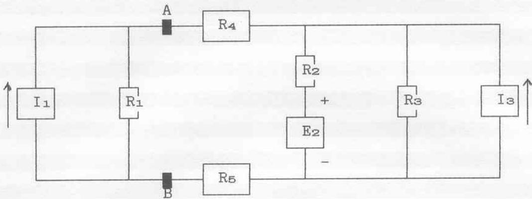
$$I_1 = 5 \text{ mA} ; \quad E_2 = 10 \text{ V} ; \quad I_3 = 2 \text{ mA} ; \quad R_1 = 2 \text{ k}\Omega$$
