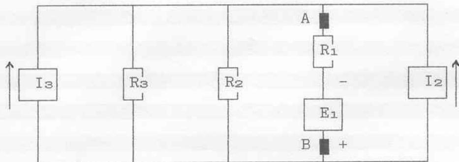
$$E_1 = 8 \text{ V} ; \quad I_2 = 10 \text{ mA} ; \quad I_3 = 5 \text{ mA} ; \quad R_1 = 3 \text{ k}\Omega$$
