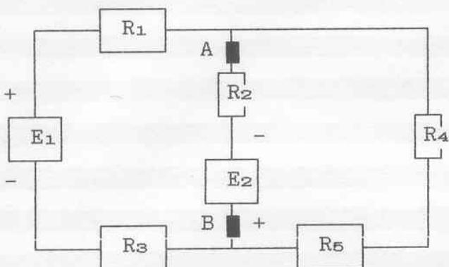
$$\begin{aligned} E_1 &= 24 \text{ V} & E_2 &= 12 \text{ V} \\ R_1 &= 1 \text{ k}\Omega & R_2 &= 1 \text{ k}\Omega \\ R_3 &= 3 \text{ k}\Omega & R_4 &= 1,5 \text{ k}\Omega \\ R_5 &= 2,5 \text{ k}\Omega \end{aligned}$$
