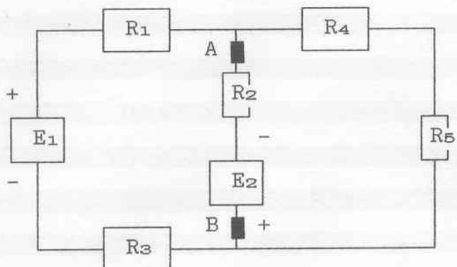
$$\begin{aligned} E_1 &= 16 \text{ V} & E_2 &= 8 \text{ V} \\ R_1 &= 2 \text{ k}\Omega & R_2 &= 2 \text{ k}\Omega \\ R_3 &= 2 \text{ k}\Omega & R_4 &= 1 \text{ k}\Omega \\ R_5 &= 1 \text{ k}\Omega \end{aligned}$$
