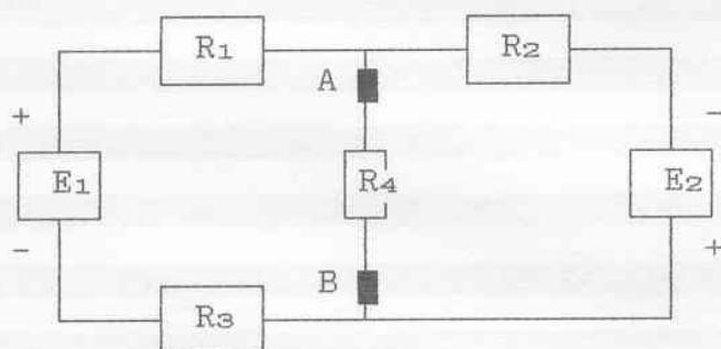
$$\begin{aligned} E_1 &= 24 \text{ V} & E_2 &= 12 \text{ V} \\ R_1 &= 1 \text{ k}\Omega & R_2 &= 2 \text{ k}\Omega \\ R_3 &= 2 \text{ k}\Omega & R_4 &= 3 \text{ k}\Omega \end{aligned}$$
