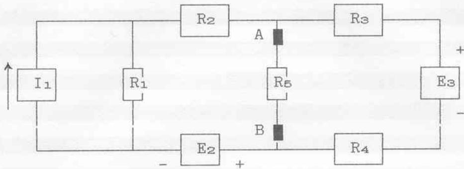
$$I_1 = 8 \text{ mA} ; E_2 = 6 \text{ V} ; E_3 = 4 \text{ V} ; R_1 = 1,5 \text{ k}\Omega$$
