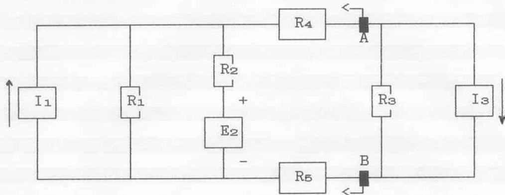
$$I_1 = 6 \text{ mA} ; E_2 = 6 \text{ V} ; I_3 = 8 \text{ mA} ; R_1 = 1,5 \text{ k}\Omega$$
