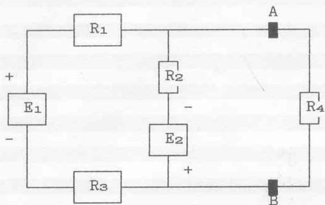
$$\begin{aligned} E_1 &= 16 \text{ V} & E_2 &= 8 \text{ V} \\ R_1 &= 2 \text{ k}\Omega & R_2 &= 2 \text{ k}\Omega \\ R_3 &= 1 \text{ k}\Omega & R_4 &= 5 \text{ k}\Omega \end{aligned}$$
