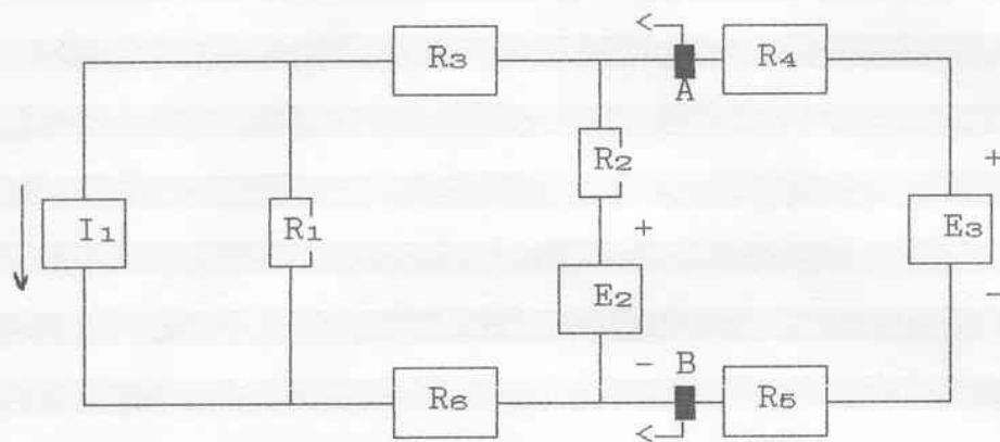
$$I_1 = 5 \text{ mA} ; E_2 = 6 \text{ V} ; E_3 = 4 \text{ V} ; R_1 = 1,6 \text{ k}\Omega ; R_2 = 1 \text{ k}\Omega$$
