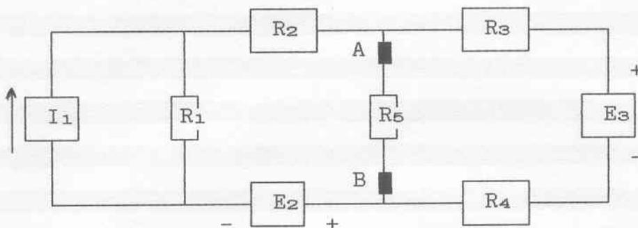
$$I_1 = 8 \text{ mA} ; E_2 = 6 \text{ V} ; E_3 = 4 \text{ V} ; R_1 = 1,5 \text{ k}\Omega$$
