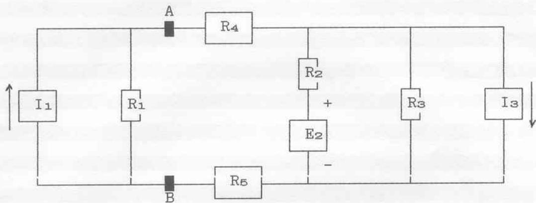
$$I_1 = 6 \text{ mA} ; E_2 = 8 \text{ V} ; I_3 = 3 \text{ mA} ; R_1 = 1 \text{ k}\Omega$$
